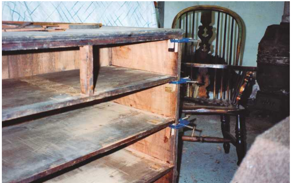
▲ Pic.1 G-clamps: the right tool for the job but keep them well padded, even on the inside of the carcass
